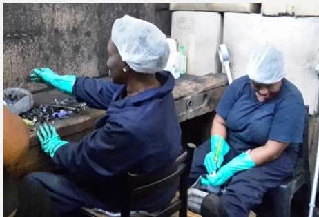
Figure 23. Dismantling of end-of-life printer cartridges for recycling
