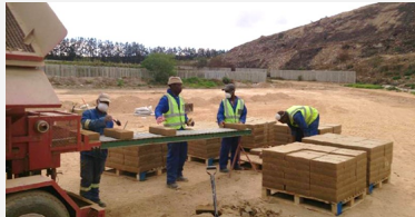
Figure 24: Compressed earth bricks manufactured from builders' rubble.
