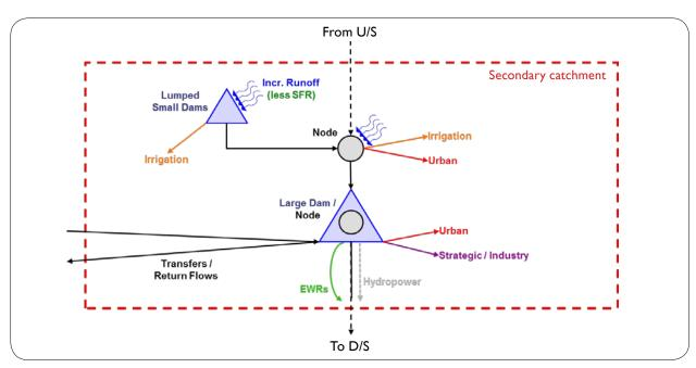
Figure 2: Generic modelling unit used for configuring the WRYM (Drawn by authors)
