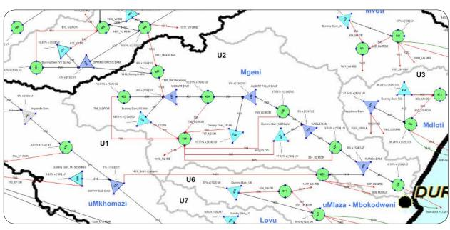
Figure 4: Details of a portion of the national WRYM system model (Mooi-Mgeni River System) (Drawn by authors)
