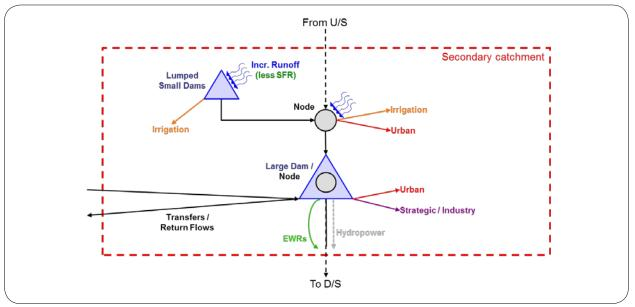
$\label{eq:Figure 4:} \qquad \mbox{Generic modelling unit used for configuration of the WRYM}$
