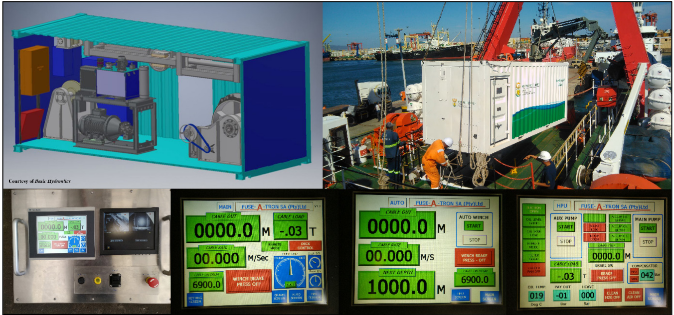
Figure 1: The top panel shows a schematic view of the containerised winch system and an image of the container being loaded onto the RV Algoa. The bottom panel shows images of the control panel and various user interface screens used during winch operations
