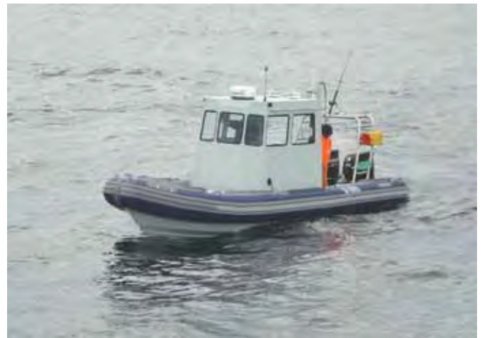
Figure 31: The acoustic survey vessel "Abyss". Equipped with state-of-the-art navigational instrumentation, acoustic equipment and long-range fuel tanks, this vessel is ideal for inshore survey work such as fish biomass estimation and the mapping of inshore habitats.
